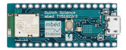
We began with a TY51822R3 BLE development board (see image) from Switch Science with a RF51822 chip from NORDIC. It has 256kB of RAM and 32kB of flash memory, is powered from the USB-B connector and has SPI, UART, I2C and GPIO ports. Then we hooked up a TMP102 temperature sensor, which communicates over the I<sup>2</sup>C port.
